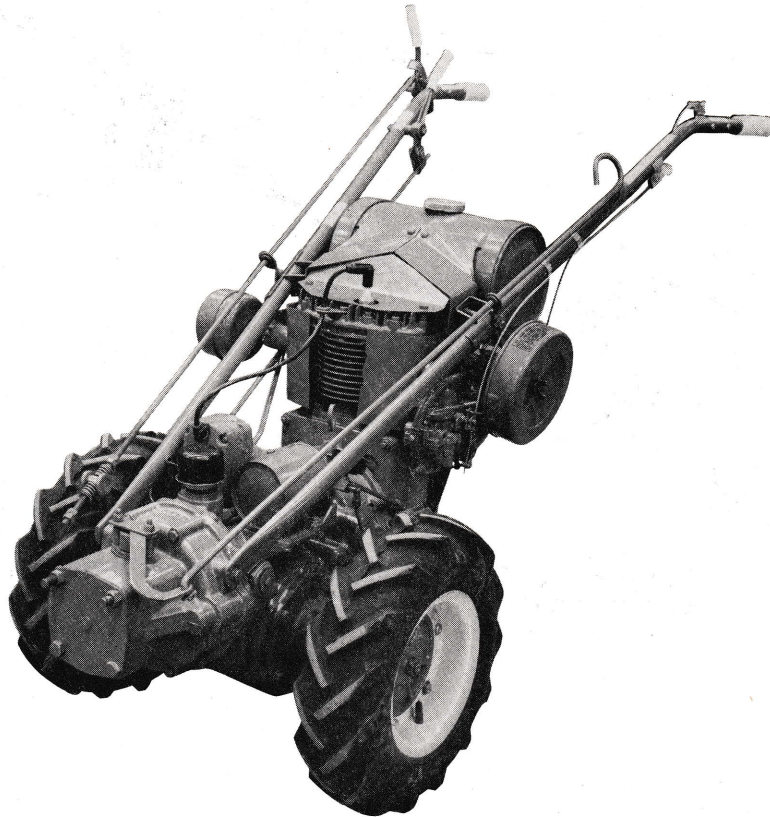
7.6 CONVERTIBLE GRAVELY EQUIPPED WITH PTO CONTROL
